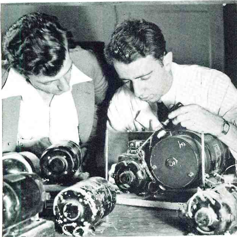
Men must study the theory and operation of motors and generators. Aircraft radio communications depend on such units for power source.
