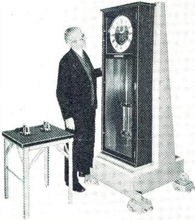
Master clock in concrete vault in the Western Union Building in New York City is precision-regulated.
