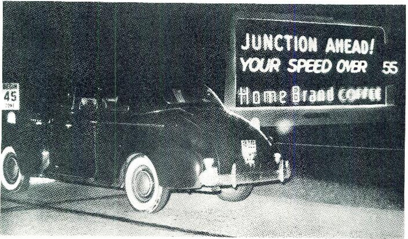
"Electronic Cop" tells motorist how fast he is going. Electronic Timer does the trick.
