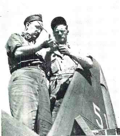
Tail end of aircraft antenna. Proper splicing is of greatest importance to prevent breakage of wires.
