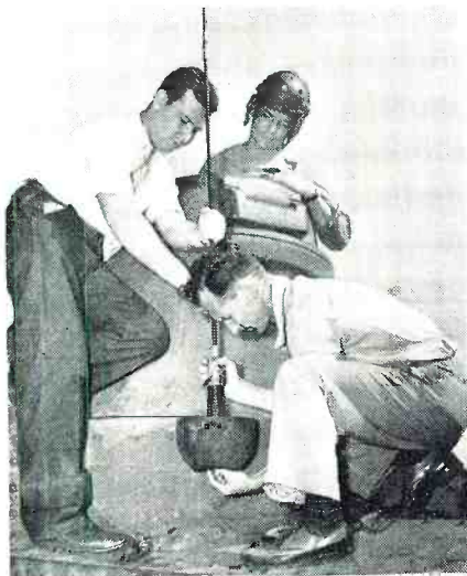
Inserting vertical tank antenna into its special insulator. Note tank helmet worn by student in rear.
